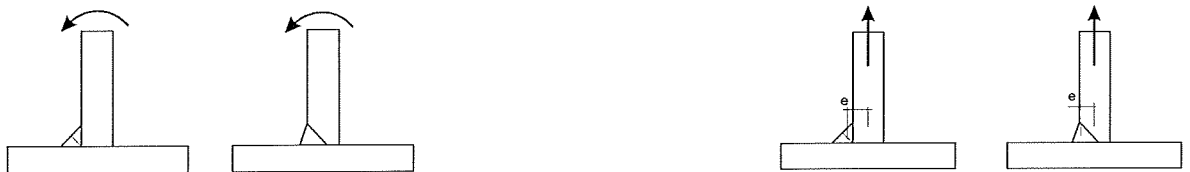
(a) Bending moment produces tension at the root of the weld. (b) Tensile force produces tension at the root of the weld.
